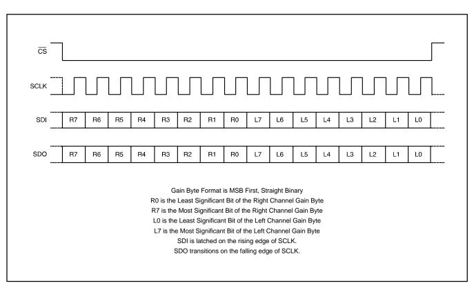
FIGURE 2: Serial Interface Protocol.
