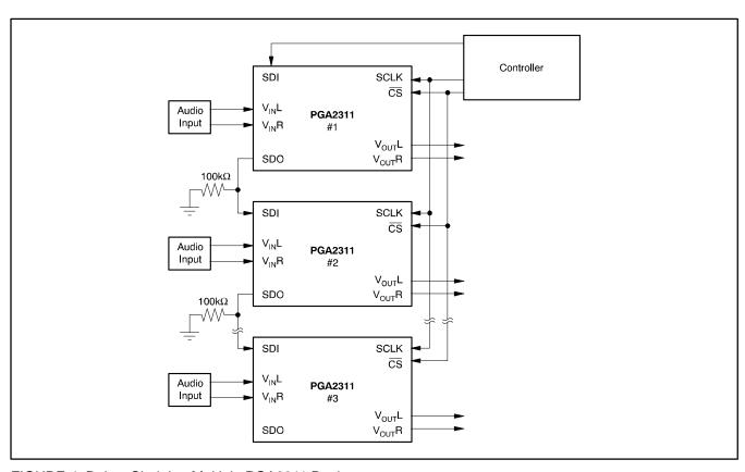
FIGURE 4: Daisy-Chaining Multiple PGA2311 Devices.
