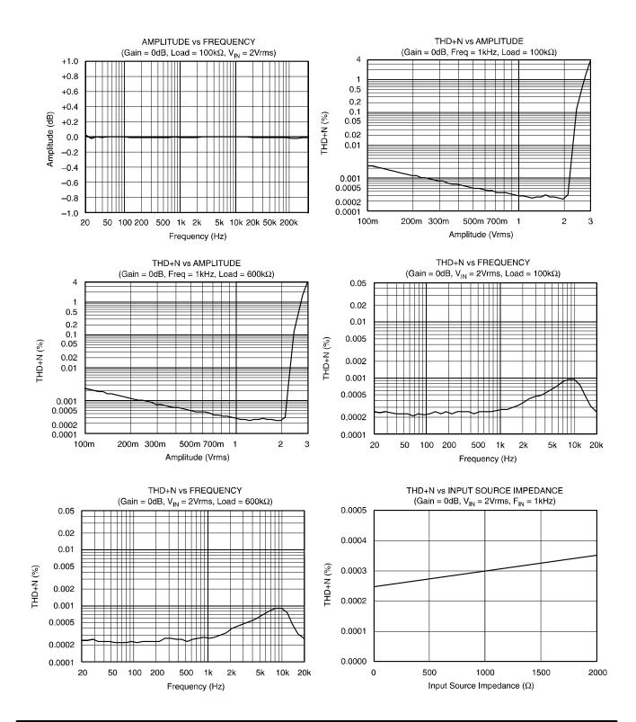
TYPICAL CHARACTERISTICS (Cont.) At  $T_A$  = +25°C,  $V_A$ + = +5V,  $V_A$ - = -5V,  $V_D$ + = +5V,  $R_L$  = 100k $\Omega$ ,  $C_L$  = 20pF, BW measure = 10Hz to 20kHz, unless otherwise noted. (NOTE: All plots taken with PGA2311 A–Grade.)
