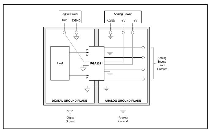
FIGURE 6: Typical PCB Layout Floor Plan.
