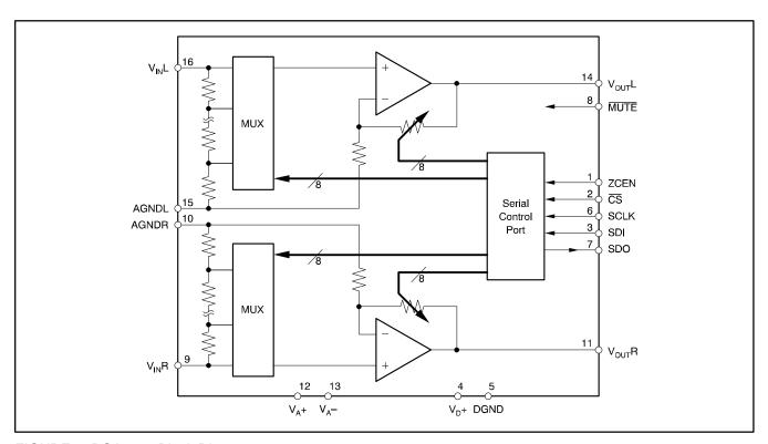
FIGURE 1: PGA2311 Block Diagram.
