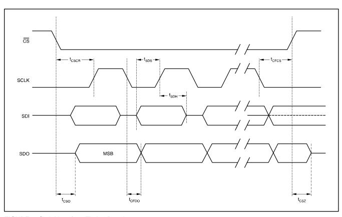
FIGURE 3: Serial Interface Timing Requirements.
