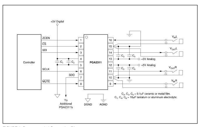
FIGURE 5: Recommended Connection Diagram.
