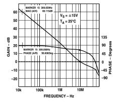
TPC 4. Open-Loop Gain, Phase vs. Frequency
