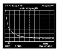
Figure 6. 1/f Noise Corner,  $V_S = \pm 15 \text{ V}$ ,  $A_V = 1000 \text{ }$
