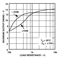
TPC 12. Maximum Output Voltage vs. Load Resistance
