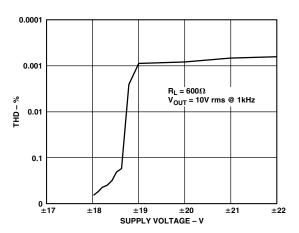
Figure 5. THD + Noise vs. Supply Voltage
