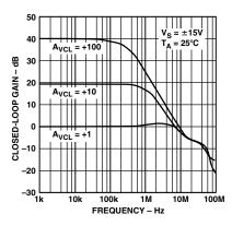
TPC 5. Closed-Loop Gain vs. Frequency
