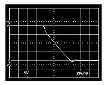
TPC 24. Negative Slew Rate  $R_L = 2 \text{ k}\Omega$  ,  $V_S = \pm 15 \text{ V}$ ,  $A_V = +1$
