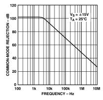
TPC 7. Common-Mode Rejection vs. Frequency
