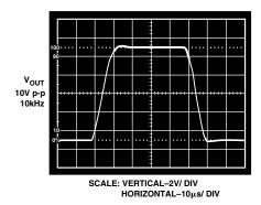
Figure 19. Low-Pass Filter Transient Response
