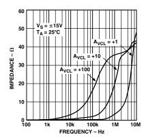
TPC 6. Closed-Loop Output Impedance vs. Frequency
