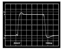
TPC 26. Small Signal Response  $R_L=2~k\Omega$  ,  $V_S=\pm 5~V$ ,  $A_V=+1$
