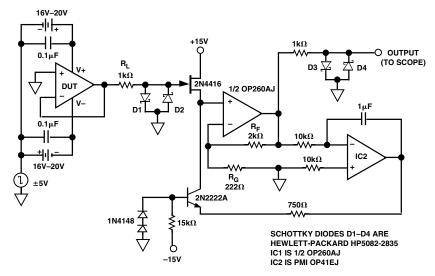
Figure 11. OP275's Settling Time Test Fixture
