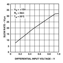
TPC 22. Slew Rate vs. Differential Input Voltage
