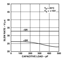
TPC 21. Slew Rate vs. Capacitive Load
