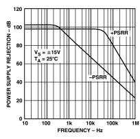
TPC 8. Power Supply Rejection vs. Frequency
