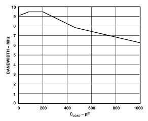
Figure 16. Bandwidth vs. C<sub>LOAD</sub>
