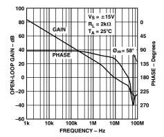
TPC 9. Open-Loop Gain, Phase vs. Frequency
