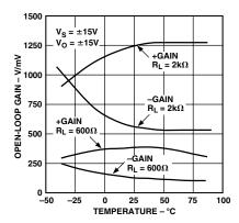
TPC 2. Open-Loop Gain vs. Temperature
