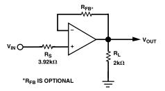
Figure 9. Output Voltage Phase Reversal Fix
