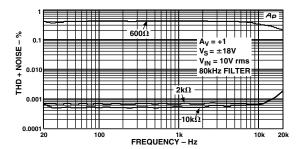
Figure 3. THD + Noise vs. R<sub>LOAD</sub>; V<sub>IN</sub> =10 V rms,
