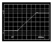
TPC 25. Positive Slew Rate  $R_L = 2 \ k\Omega$  ,  $V_S = \pm 15 \ V$ ,  $A_V = +1$
