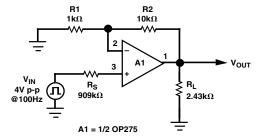
Figure 10. Overload Recovery Time Test Circuit
