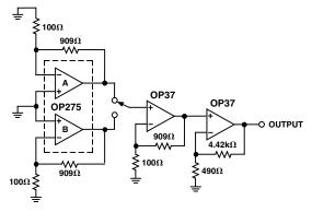
Figure 7. Noise Test Fixture
