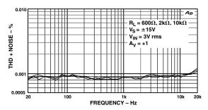
Figure 2. THD + Noise vs. Frequency vs. R<sub>LOAD</sub>
